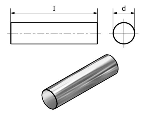
$\begin{array}{ll} \text{d1} & = 8 \\ \text{I} & = 32 \\ \text{Nominal adhesive forces} = 3.8 \\ \text{Weight in g} & = 450 \end{array}$
